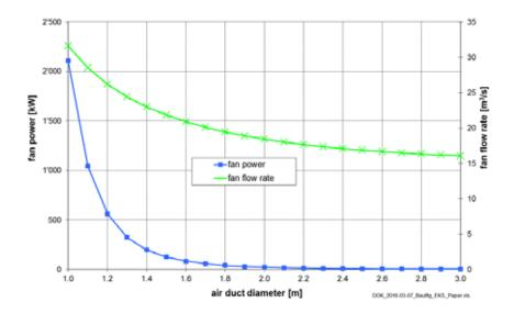
**Figure 5:** Calculated, possible fan power and flow rate vs air duct diameter for a given fresh air supply at tunnel face (12.5 m<sup>3</sup>/s), ventilation of exploratory tunnel section (about 8 km), construction lot Wolf (first construction phase).
