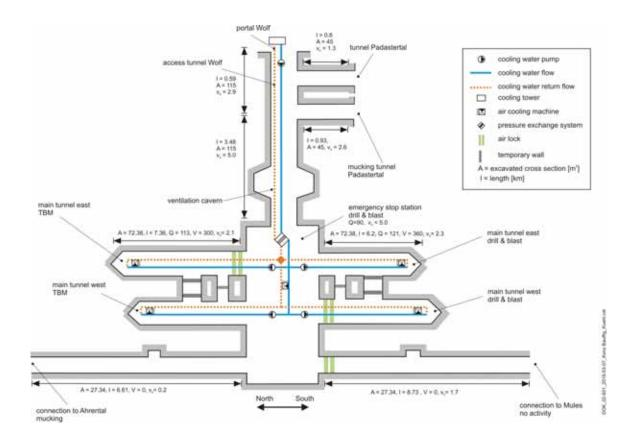
Figure 4: Cooling concept construction lot Wolf.
