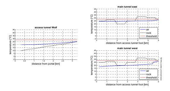
Figure 6: Calculated temperature along access tunnel and main tunnels south, construction lot Wolf.
