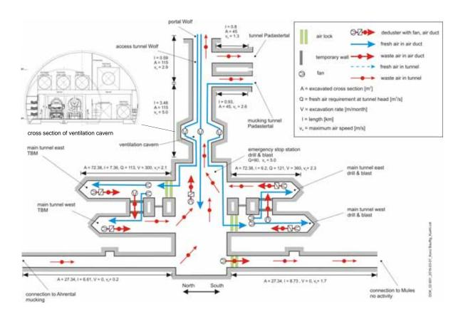
Figure 3: Ventilation concept construction lot Wolf.
