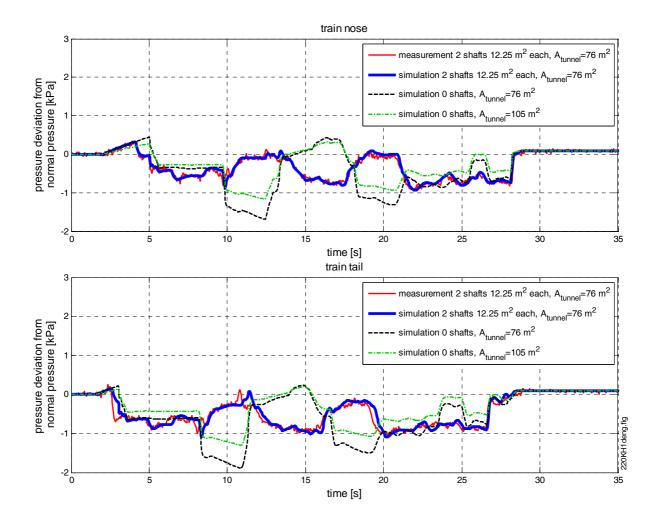
Figure 6: Simulated and measured pressure deviation from normal pressure close to the train nose and tail ( $v_{train} = 220 \text{ km/h}$ )
