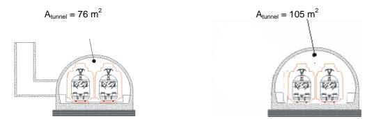
Figure 8: Measures to reduce pressure fluctuation in the Emmequerung tunnel in order to comply with the pressure comfort criterion (left: 2 pressure relief shafts each 12.25 m<sup>2</sup>, tunnel cross-section  $A_{tunnel} = 76$  m<sup>2</sup>, right: increased tunnel cross-section  $A_{tunnel} = 105$  m<sup>2</sup>, no pressure relief shaft).
