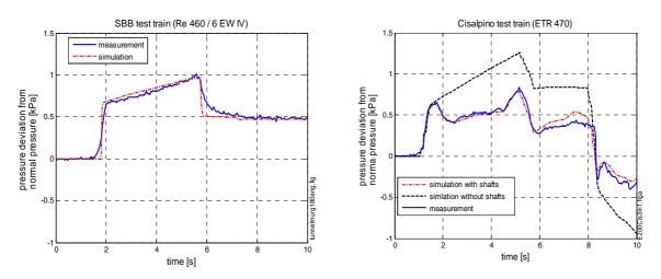
Figure 5: Pressure signals from Murgenthal tunnel (left hand, no pressure relief shafts) and from Emmequerung tunnel (right hand, two pressure relief shafts)
