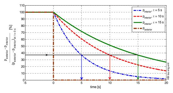
Figure 1: Pressure development in train for a sudden pressure difference to the exterior at t = 0 s ( $\tau = 5$ , 10 and 15 s)
