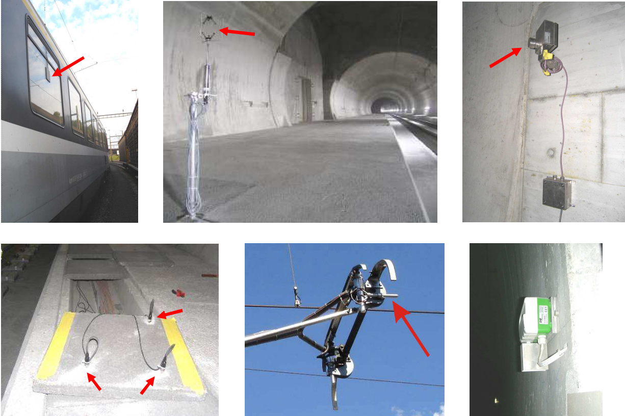
Figure 2 - Pressure transducer on window of train; 3-axis anemometer on sidewalk in cross-over; 1-d ultrasonic anemometer in single track tunnel; micro-accelerometers underneath cover plate of cable tray of sidewalk; Prandtl's pitot tube at pantograph of train; temperature and humidity sensor in single track tunnel
