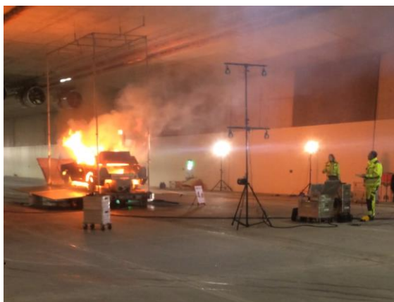
Fire test to verify airflow and smoke propagation velocities
