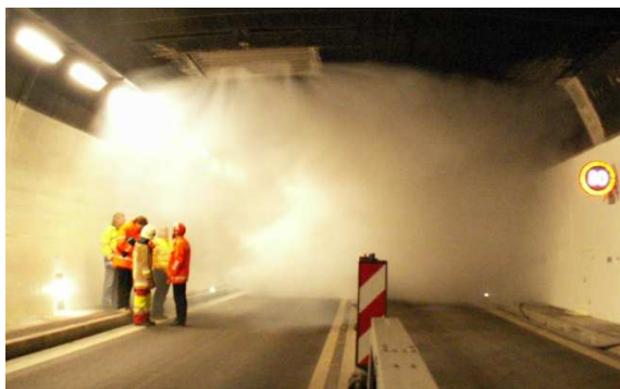
Smoke extraction tests in the Loppertunnel
