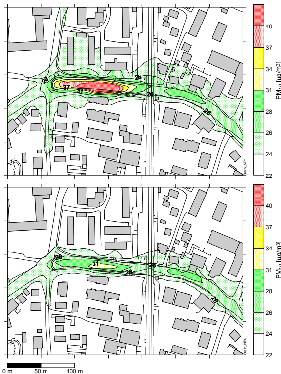
2012 annual mean of PM10-concentration at the northern tunnel portal without (above) and with (below) air extraction; MISKAM simulation
