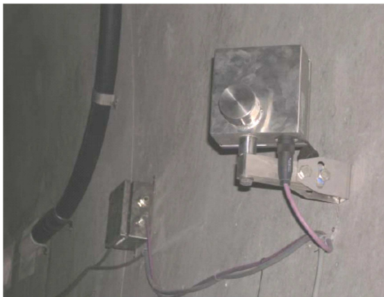
Aerodynamic acceptance measurements (1D ultrasound flow measurement system for non-contact measurement of the flow speed)
