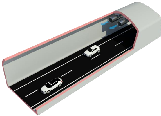
Jet fans in a tunnel cross section
