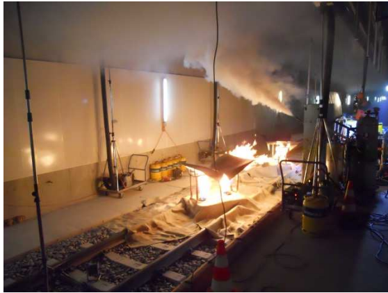
Real fire test and fume layer at the source of the fire
