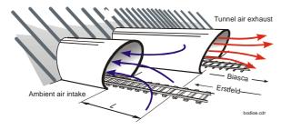
Staggered arrangement of portals for reducing air recirculation, i.e. the intake of warm and humid waste air from the exit tube into the entrance tube is reduced
