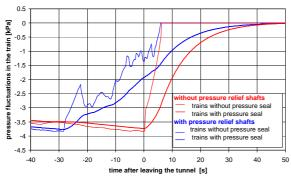
Pressure fluctuation in a passenger train leaving the
