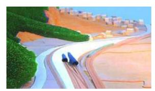
Model for the optimisation of the position of portals in the wind tunnel
