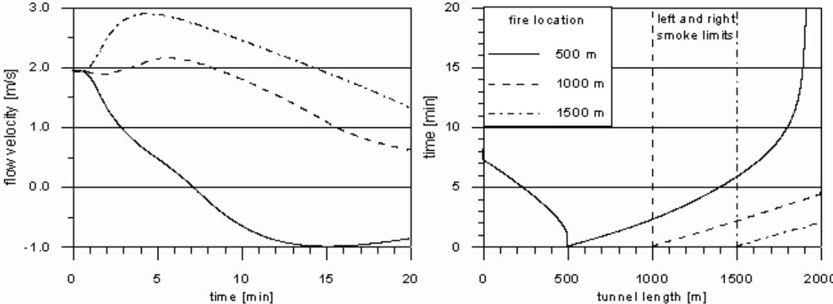
Figure 2: Flow velocity and smoke limits for a fire in a 2000 m tunnel with two-way traffic at 60 km/h, three fire locations and a traffic distribution of 600/300 veh/h.
