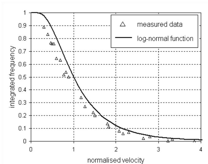
Figure 5: Typical distribution of wind velocities, normalised with the average velocity [8].
