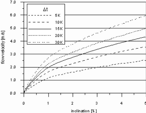
Figure 3: Flow velocity in a 2000 m tunnel versus tunnel inclination as a function of the temperature difference  $\Delta t$ .
