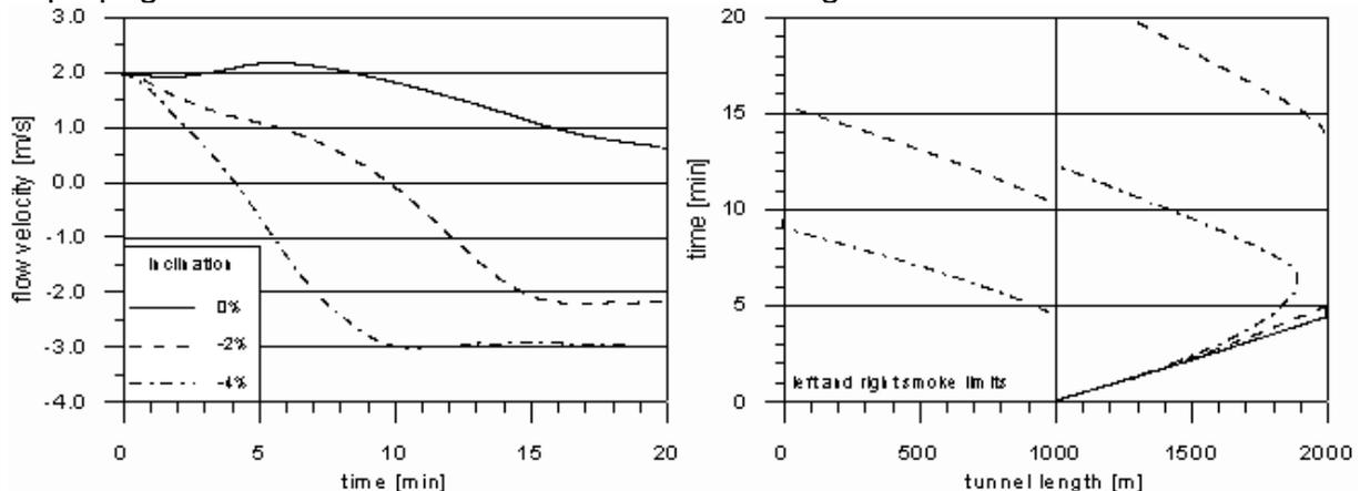
Figure 4: Flow velocity and smoke limits for a 20 MW fire, two-way traffic, 600/300 veh/h at 60 km/h, fire location at  $x=1000$  m.
