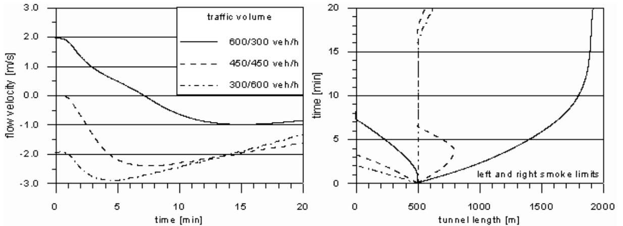
Figure 1: Flow velocity and smoke limits for a 20 MW fire located at  $x = 500$  m, the vehicle speed was 60 km/h and the traffic distributions varied.
