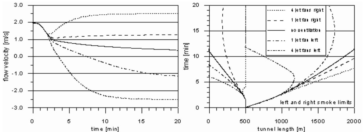
Figure 6: Flow velocity and smoke limits for a fire in a 2000 m tunnel, 600/300 veh/h at 60 km/h and different ventilation strategies.
