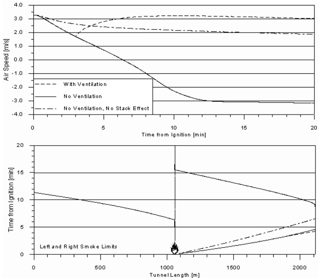
Figure 6: Air speed and smoke limits for a 20 MW fire in the Pierre Pertuis tunnel (uni-directional traffic, 270 veh/h; vehicle motion from left to right).
