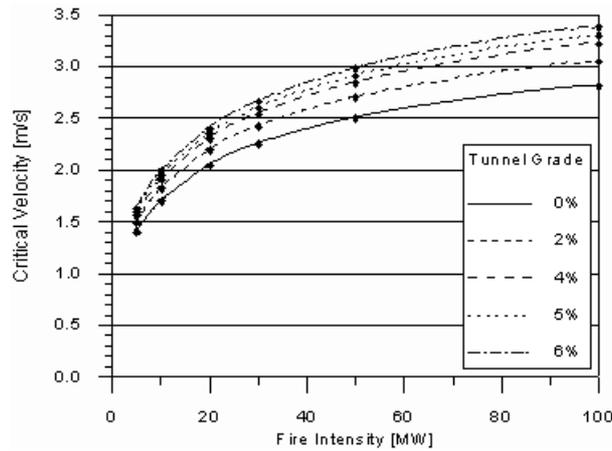
Figure 4: Critical velocity vs. fire intensity and tunnel inclination (grade).
