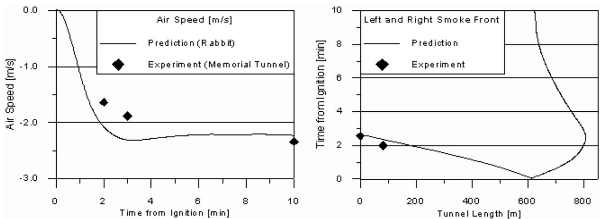
Figure 3: Memorial Tunnel test number 502: natural ventilation with fire intensity 50 MW.
