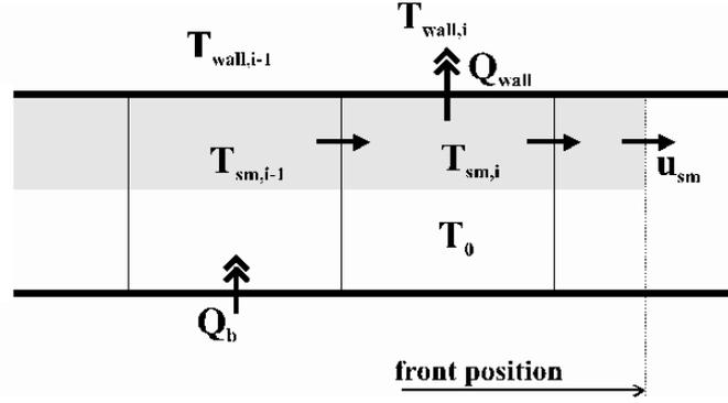
Figure 2: Model for the propagation of the smoke layer.
