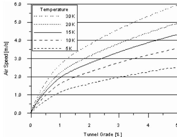
Figure 5: Air speed vs. tunnel inclination (grade) and mean temperature in the tunnel.
