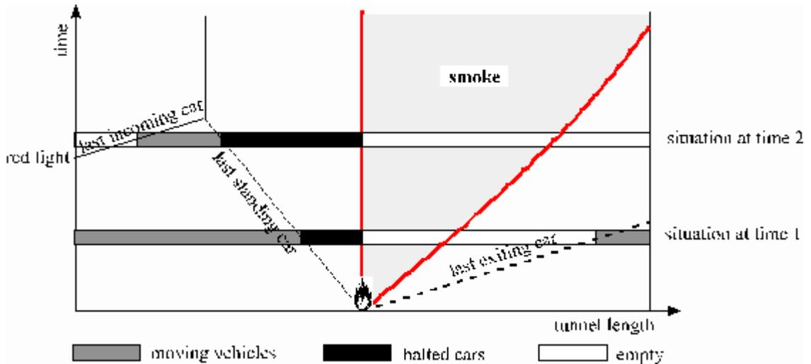
Figure 1: Time dependent traffic distribution and smoke propagation from the start of the fire [4]
