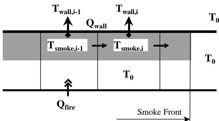
Figure 5: Model for the heat fluxes as modelled in Sprint [4]
