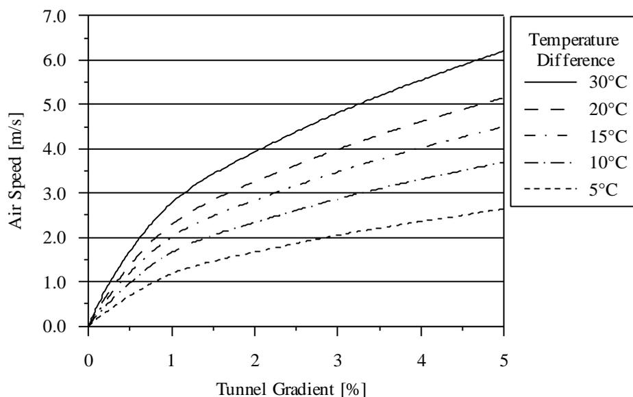
Figure 1: Air speed vs. tunnel gradient and temperature difference in a 3000 m long tunnel
