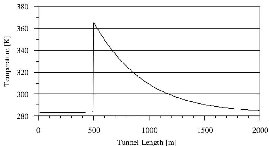
Figure 7: Temperature distribution in the vicinity of the fire,  $t = 10$  min, fire load 30 MW, tunnel length 2000 m, 5% gradient, without traffic and mechanical ventilation
