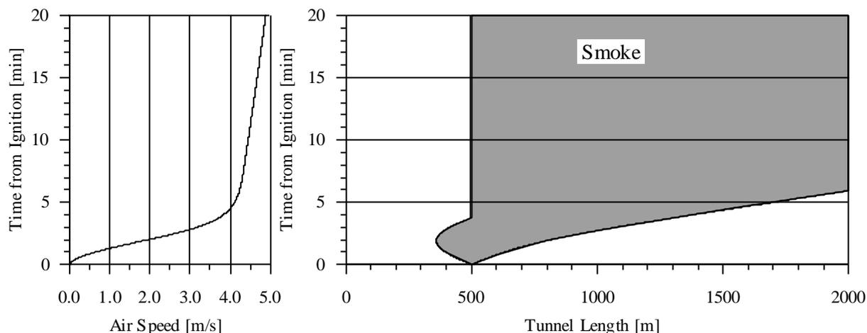
Figure 6: Flow velocity and smoke propagation in the tunnel, fire load 30 MW, tunnel length 2000 m, 5% gradient from left to right, without traffic and mechanical ventilation
