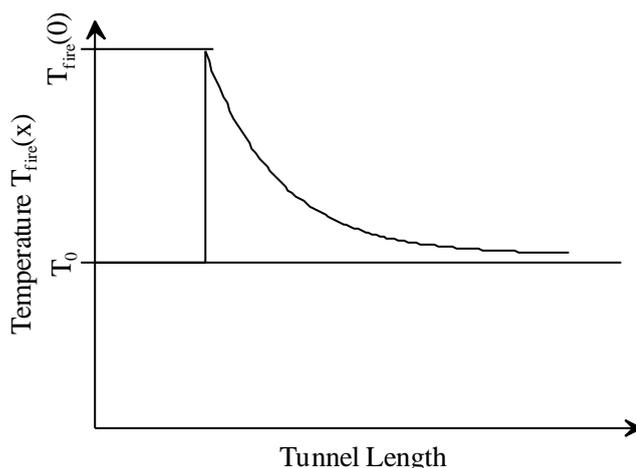
Figure 4: Temperature distribution in the vicinity of the fire according to the model [3]
