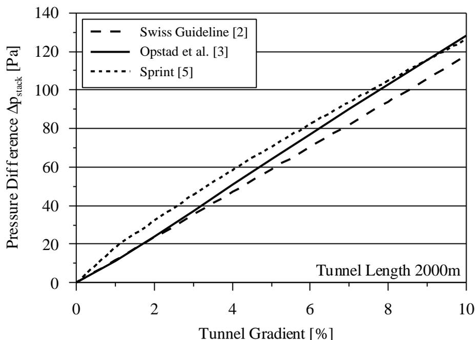
Figure 8: chimney effect versus tunnel gradient, tunnel length 2000 m, fire load 30 MW
