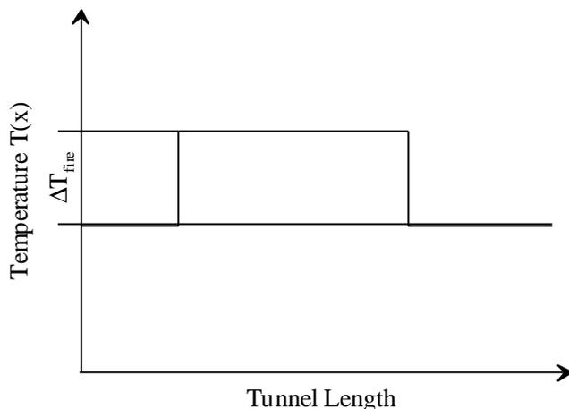
Figure 2: Idealised temperature distribution in the vicinity of the fire, Swiss guideline [2]
