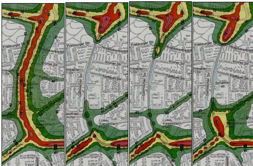
Figure 1: Mittlerer Ring southwest - Annual mean concentration of  $\text{NO}_2$ , situation without tunnel and with three different tunnel designs, year 2010.
