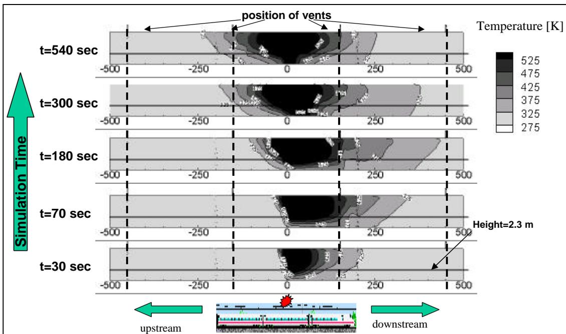
**Figure 8 Transient development of the temperature in a section plane parallel to the train at a distance of 0.75 from the tunnel wall (representative for the situation on the emergency walkway - highest shown temperature is 525 K )**
