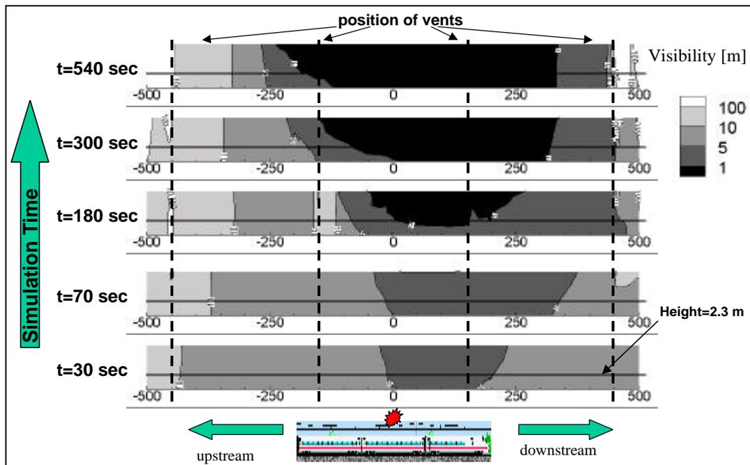
**Figure 9** Transient development of the visibility in a section plane parallel to the train at a distance of 0.75 from the tunnel wall (representative for the situation on the emergency walkway)
