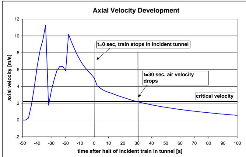
The development of the axial velocity upstream of the fire is shown in Figure 4. The entering train induces air velocity with a peak level of approximately 10 m/s in the tunnel. After halt of the train, the velocity decreases quickly. The velocity drops below the predicted critical velocity (2.2 m/s see Chapter 3.2) after about 30 sec
