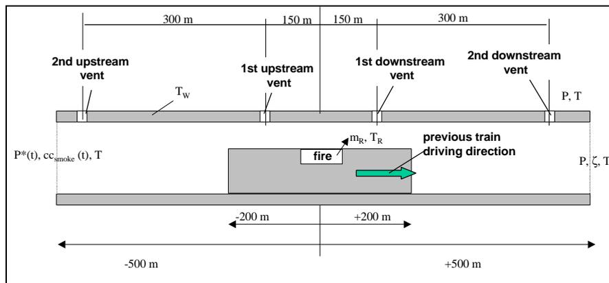
**Figure 2 Computational Domain for CFD simulation**
