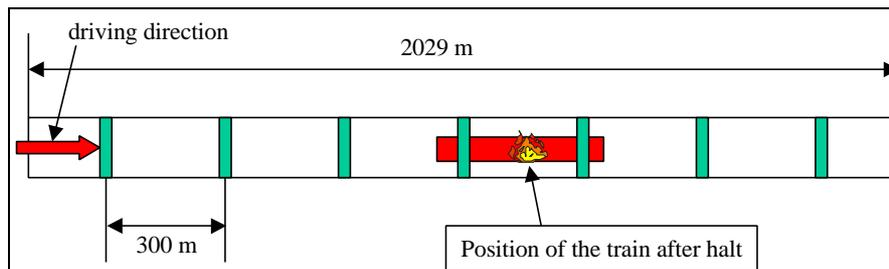
**Figure 1 Geometry of the tunnel and position of the train after halt in the tunnel**
