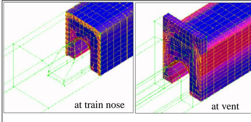
A state-of-the-art hybrid meshing technique was used to efficiently mesh the geometry. The grid consists of 180'000 cells with variable shape: hexahedral, pyramidal and tetrahedral. Grid refinement was used in important areas near the tunnel walls. Details are shown in Figure 3
