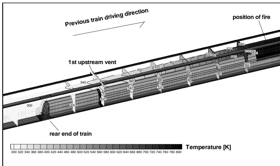
**Figure 7** Temperature distribution near the train upstream of the fire at 280 sec after halt of the train
