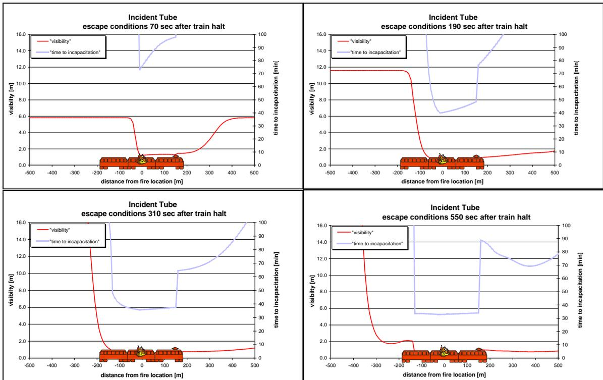
**Figure 6** Visibility and time to incapacitation at 70, 190, 310, 550 sec after halt of the train
