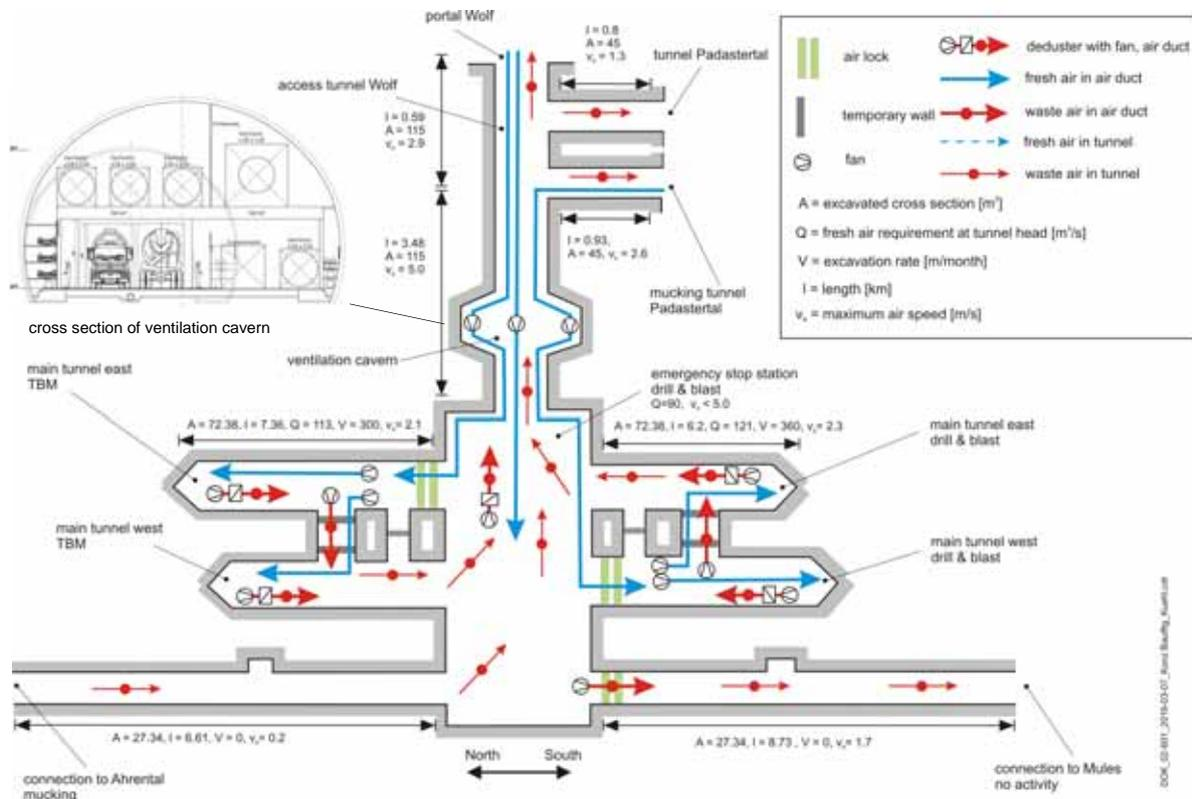
Figure 3: Ventilation concept construction lot Wolf.
