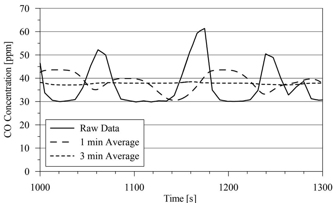
Figure 6: Calculated CO Level at the Exit Portal, Raw Data at 18 km h<sup>-1</sup> and Running Average
