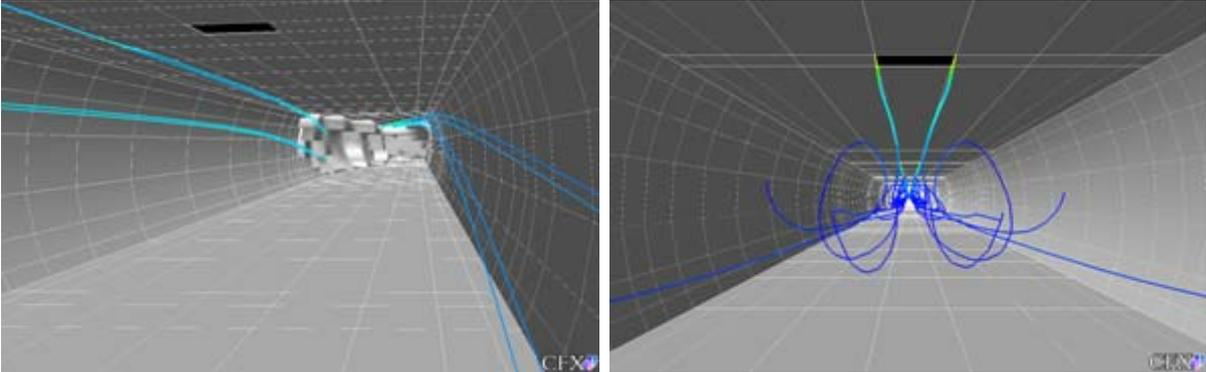
*Fig. 10 Left hand picture: Streamlines departing from dampers 54 and 55. Position of the observer: 225 m from the fire source, looking east; Right hand picture: Streamlines departing from various dampers. Position of the observer: 600 m from the east portal, looking west.*
