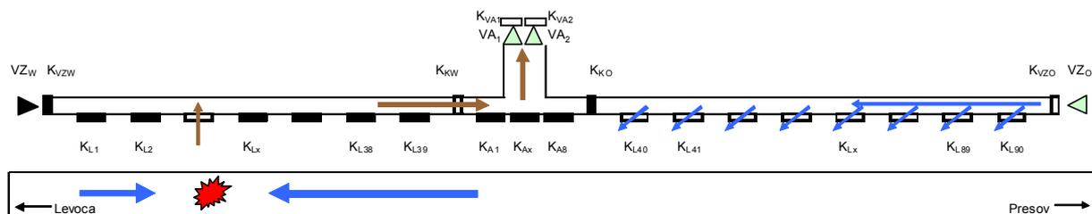
Fig. 3 Main response mode of the ventilation system in case of a fire
