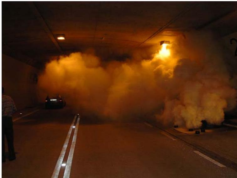
*Fig. 12 Fog grenades producing smoke*
