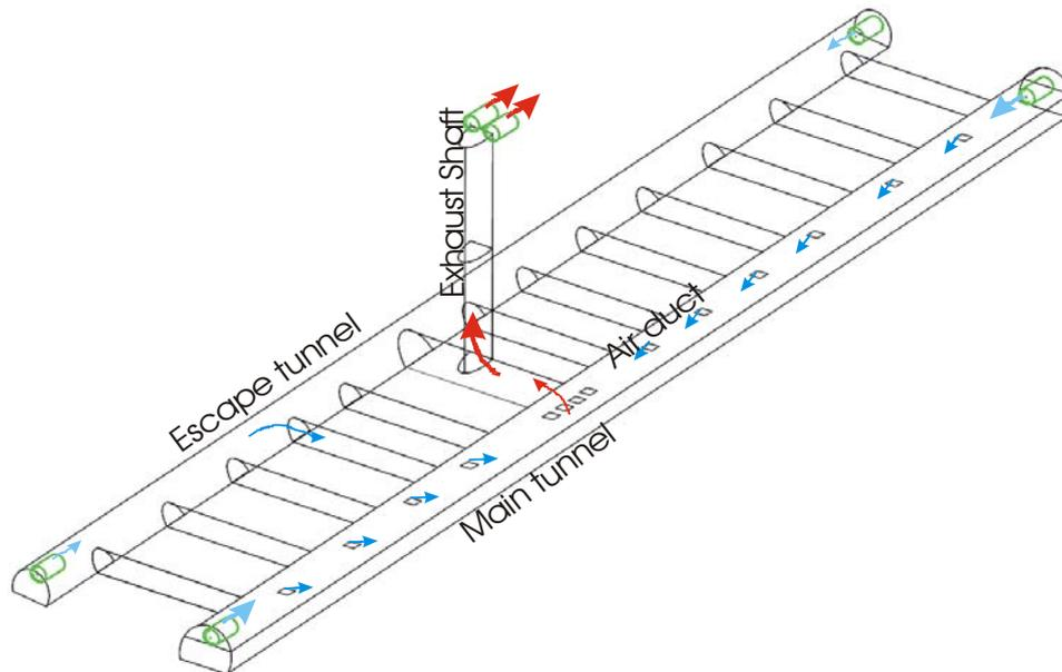
Fig. 1 Overview of the tunnel with its ventilation system
