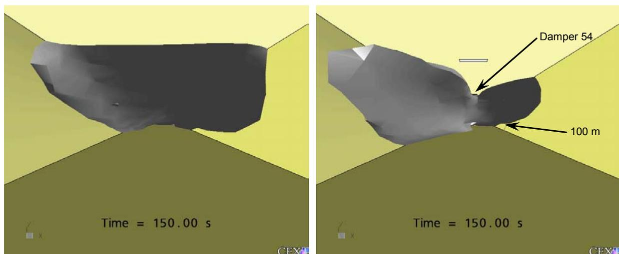
*Fig. 9 Smoke stratification of the 30 MW fire at  $t=150$  s. Ventilation modes: extraction (left hand picture) and extraction with semi-transverse ventilation (right hand picture). Position of observer: 180 m from the fire source, looking east.*
