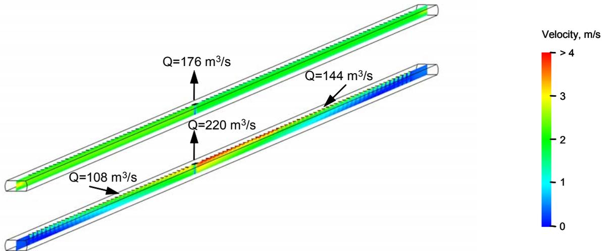
*Fig. 6 Velocities in the tunnel resulting from the ventilation mode and the specified volume flows: extraction (above) and extraction together with semi-transverse ventilation (below)*
