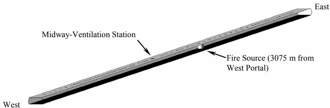
Fig. 5 Domain used for CFD Computations (entire tunnel)
