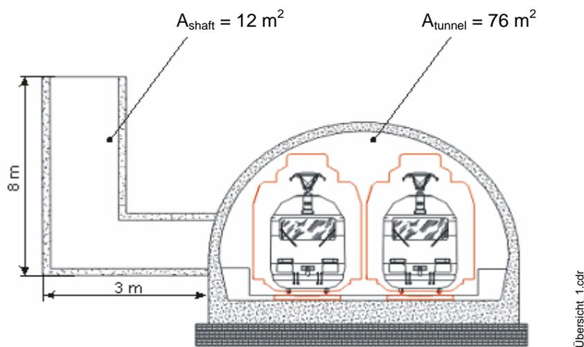
**Figure 3: Schematic view of the cross-section of the Emmequerung tunnel with a pressure relief shaft**
