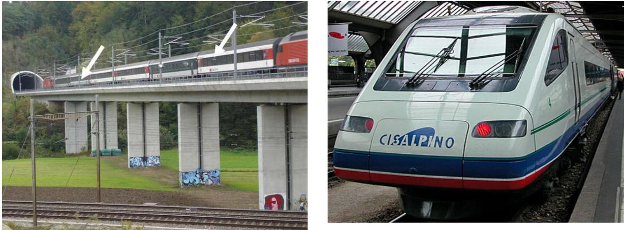
**Figure 4: Trains for the measurements (left hand: SBB test train at east portal of the Murgenthal tunnel, white arrows indicate the pressure measuring positions, right hand: Cisalpino test train)**
