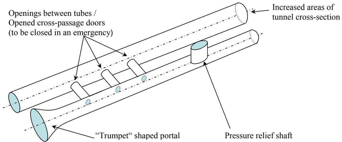
**Figure 2: Measures in tunnels in order to decrease the pressure fluctuations**
