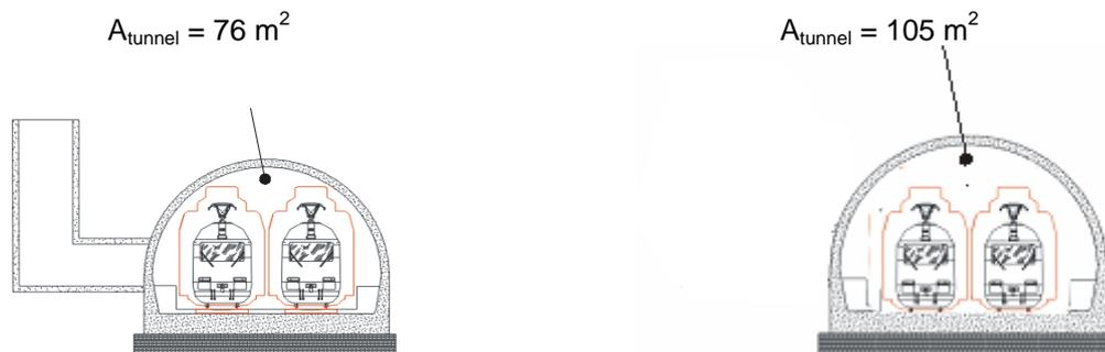
**Figure 8: Measures to reduce pressure fluctuation in the Emmequerung tunnel in order to comply with the pressure comfort criterion (left: 2 pressure relief shafts each 12.25 m<sup>2</sup>, tunnel cross-section  $A_{\text{tunnel}} = 76 \text{ m}^2$ , right: increased tunnel cross-section  $A_{\text{tunnel}} = 105 \text{ m}^2$ , no pressure relief shaft).**
