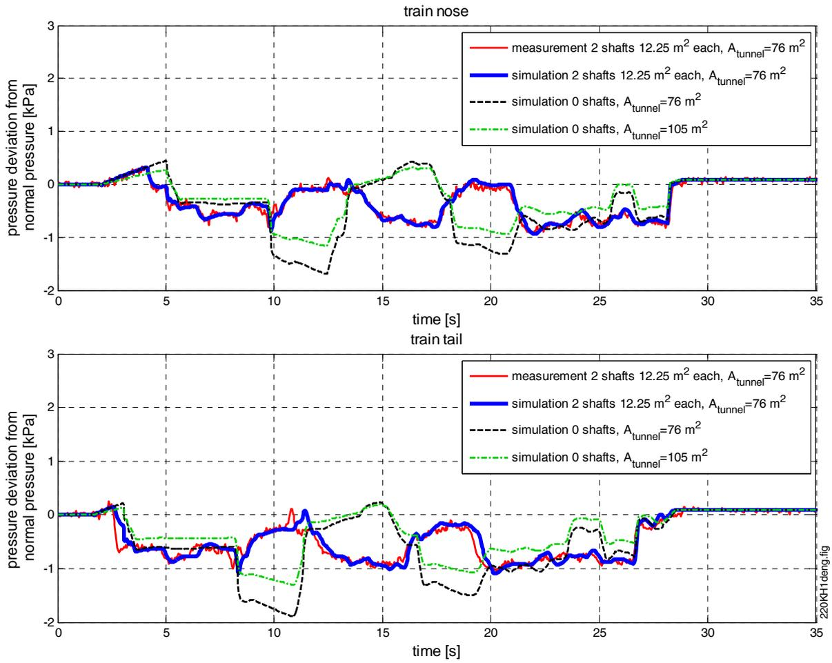
**Figure 6: Simulated and measured pressure deviation from normal pressure close to the train nose and tail ( $v_{\text{train}} = 220 \text{ km/h}$ )**
