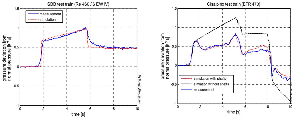
**Figure 5: Pressure signals from Murgenthal tunnel (left hand, no pressure relief shafts) and from Emmequering tunnel (right hand, two pressure relief shafts)**
