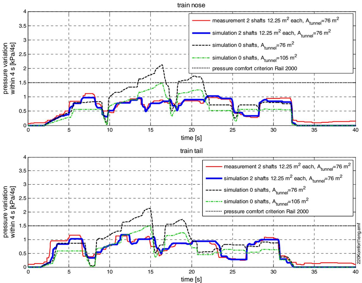
**Figure 7: Measurement and simulation for Emmequerung tunnel (2 shafts and without shafts) of pressure variation in 4 s compared to pressure comfort criterion**
