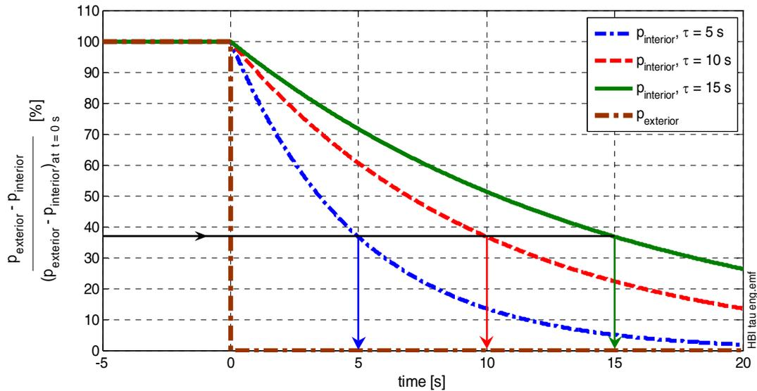
**Figure 1: Pressure development in train for a sudden pressure difference to the exterior at  $t = 0$  s ( $\tau = 5, 10$  and  $15$  s)**
