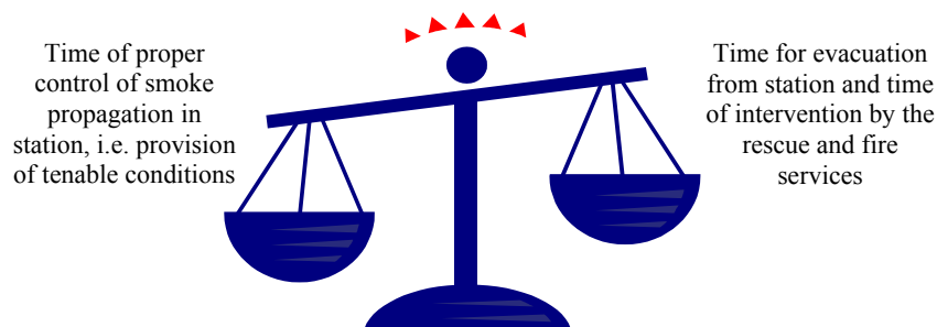
Figure 1. Balance between time for self-rescue and time for proper control of smoke
