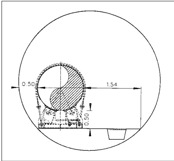
Cross-section of the 3800 mm diameter tunnel with the gas pipe line; units m
