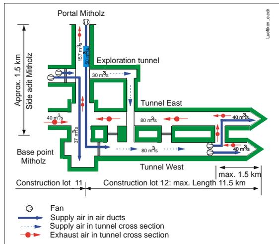
Ventilation system in the intermediate access at Mitholz
