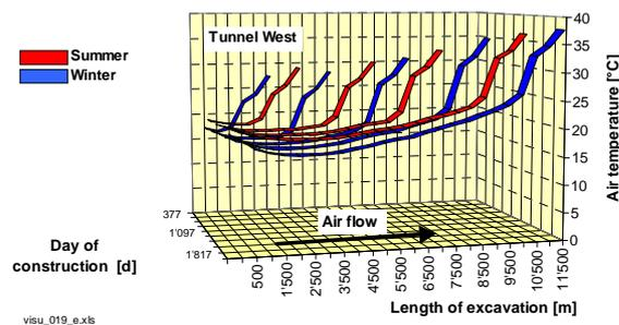
Calculated air temperatures according to excavation progress without cooling
