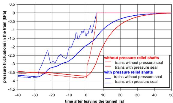
Pressure fluctuation in a passenger train leaving the tunnel
