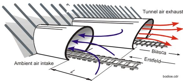
Staggered arrangement of portals for reducing air recirculation, i.e. the intake of warm and humid waste air from the exit tube into the entrance tube is reduced
