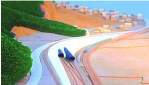
Model for the optimisation of the position of portals in the wind tunnel
