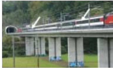
Left hand: Train for aerodynamic measurements equipped with pressure sensing devices (white arrows); Right hand: Double-deck IC-trains – Study of their effect on landside infrastructure, pressure fluctuations in tunnels and their sensitivity to side-winds
